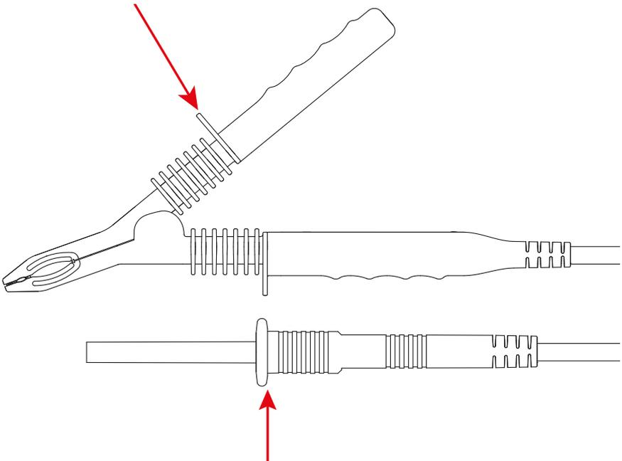
Measurements of voltages  $\geq 1000$  V on supply lines should be made using the test probes only, with the user's hands behind the hand guard on the lead.
