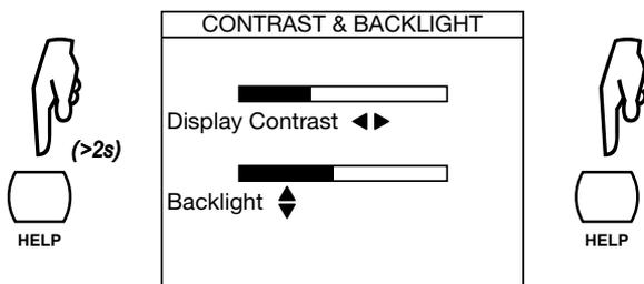
These adjustments are stored even after the instrument is switched off.
