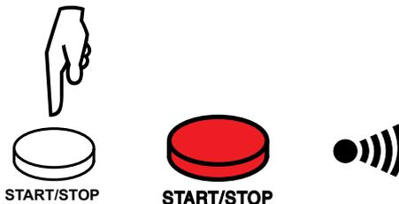
If the test voltage generated is >5000 V, the **START/STOP** button blinks.
