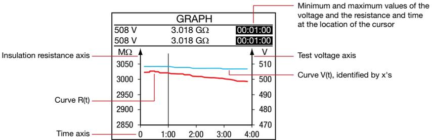
This curve is plotted using samples recorded during the measurement.
