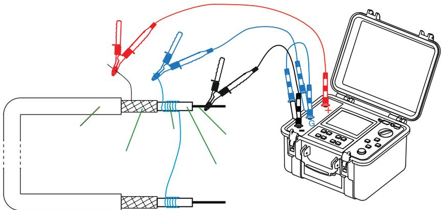
Using the guard eliminates the influence of the surface leakage current. A conducting wire must be wrapped around the insulation.
