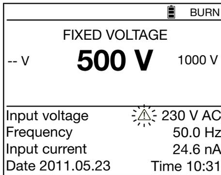
When the external voltage exceeds 25 V, the blinking (
