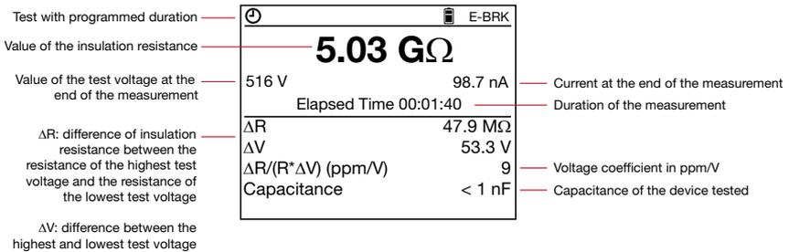
Record the measurement and compare it to earlier measurements in order to assess the evolution of its value. Also record the temperature and the ambient relative humidity.
