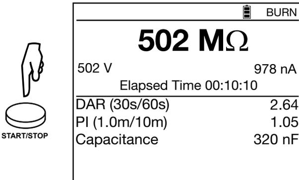
*\*The terms DAR, PI, DD and the capacity and current leak measurements are included in the quantity **MΩ**.*
