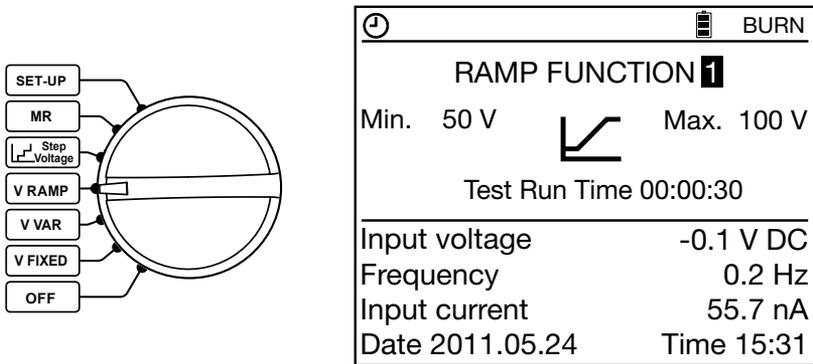
Use the ▲ ▼ buttons to select a preset test voltage ramp:
