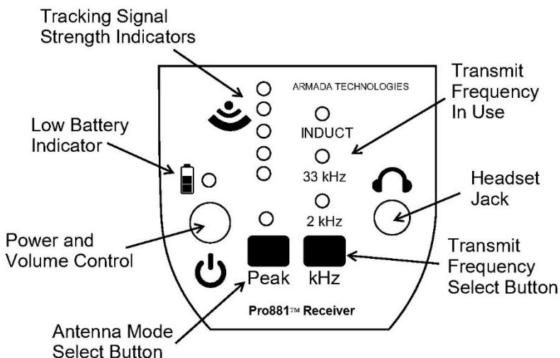
**Receiver Operation** – Turn on your receiver by turning the volume control clockwise. Once again, battery condition is indicated by the light directly above the power dial (light off = good battery, light on = low battery).
