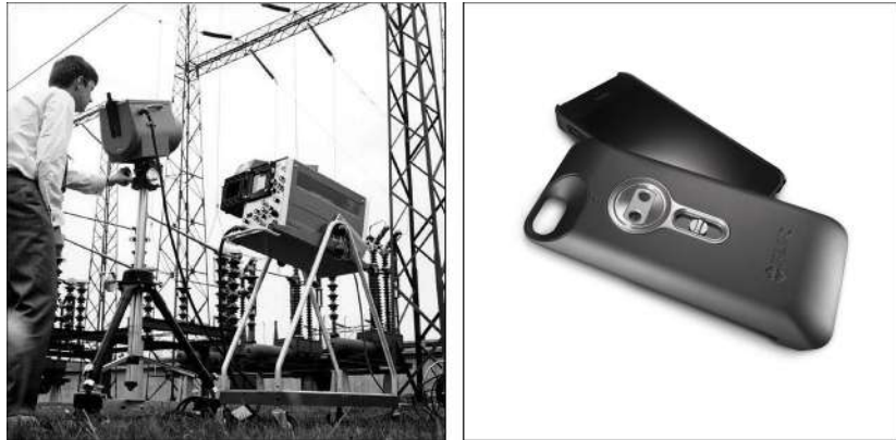
Figure 13.2 LEFT: Thermovision Model 661 from 1969. The camera weighed approximately 25 kg (55 lb.), the oscilloscope 20 kg (44 lb.), and the tripod 15 kg (33 lb.). The operator also needed a 220 VAC generator set, and a 10 L (2.6 US gallon) jar with liquid nitrogen. To the left of the oscilloscope the Polaroid attachment (6 kg/13 lb.) can be seen. RIGHT: FLIR One, which was launched in January 2014, is a slide-on attachment that gives iPhones thermal imaging capabilities. Weight: 90 g (3.2 oz.).
