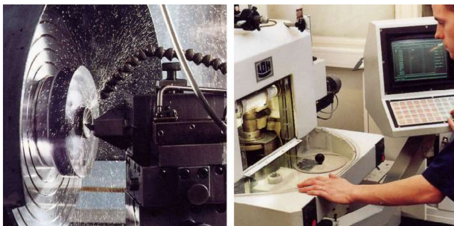
Figure 13.4 LEFT: Diamond turning machine; RIGHT: Lens polishing
