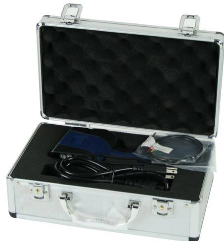
ST-5100 with included carrying case, charger and sensor connection cable.
