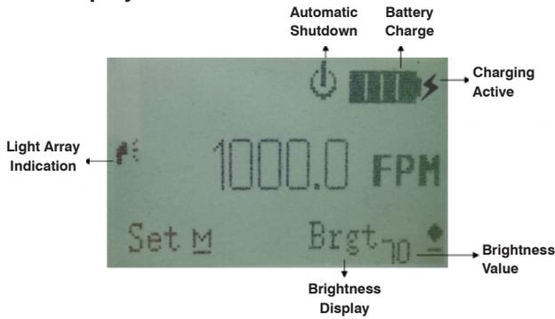
Automatic Power Off icon appears at top if selection is set for unit to have 10 minute auto-shut off active.
